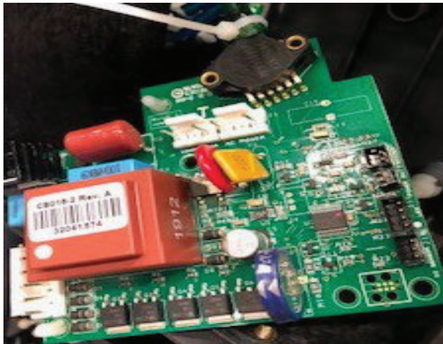
Figure 13. Pressure sensor tubing reconnected to board with zip tie.
