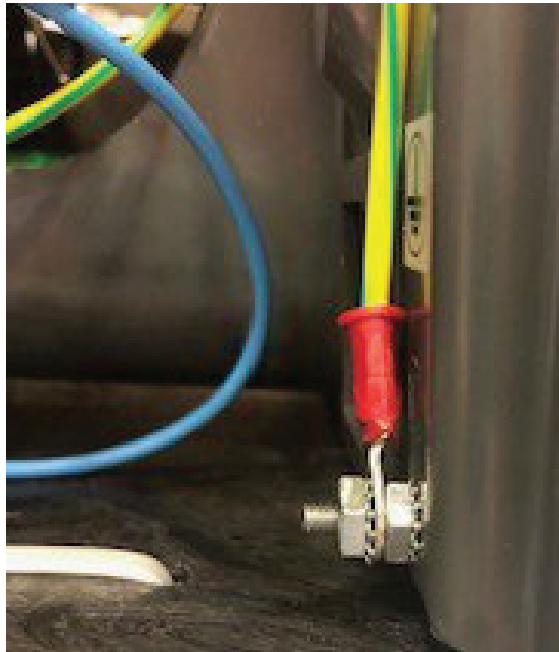
Figure 25. Showing ground wire and nut re installed.
