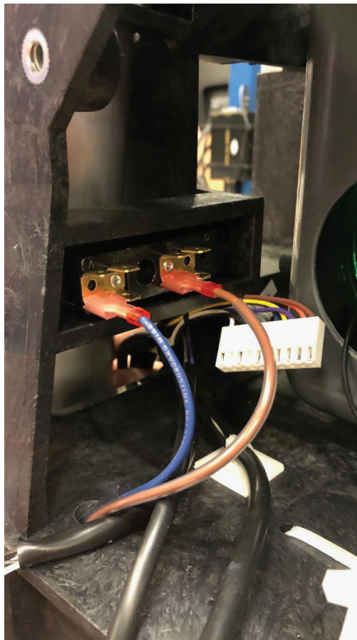
Figure 6. Terminal block with only blue and brown compressor wires.
