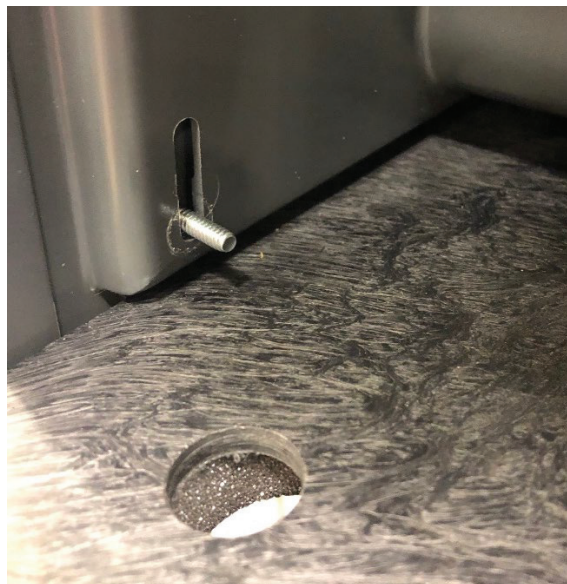
Figure 11. Shows the screw on the front panel once the nut is removed.
