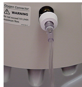
Figure 10: DISS Nut and Tailpiece connected to Reservoir Outlet
