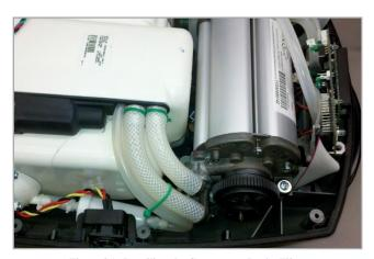
Figure 25: Installing the Compressor Intake Filter.
