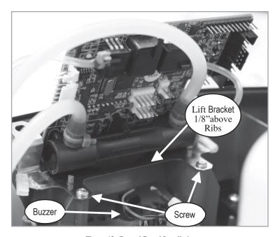
Figure 43: Control Board Installation.
