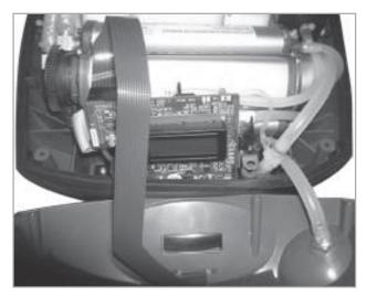
Figure 26: Membrane Panel Ribbon Cable Installation.
