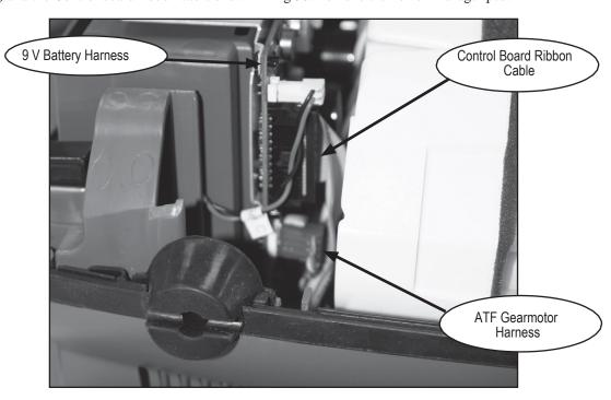
Fig 50: Wire harnesses and control board ribbon
