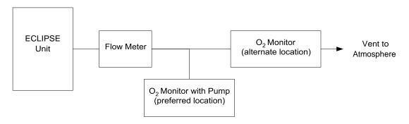
Figure 27: CAIRE Recommended Test Setup to verify performance of Oxygen Concentrator
