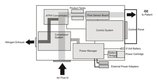
Figure 1: Eclipse 5 System Block Diagram
