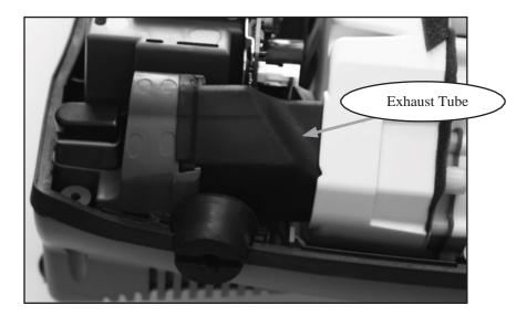
Fig 49: Exhaust Tube
