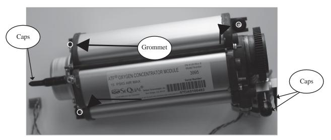
Figure 34: ATF Module Grommet Installation
