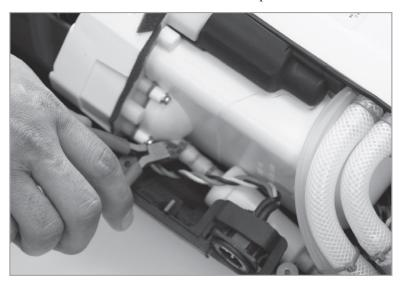
Figure 24: Removing the Compressor Intake Filter.
