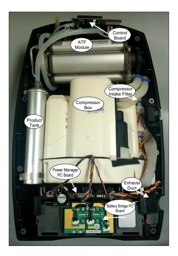
Figure 30: Bottom Case Components
