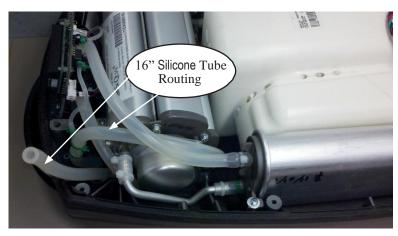
Figure 35: Tube Routing under ATF Module.
