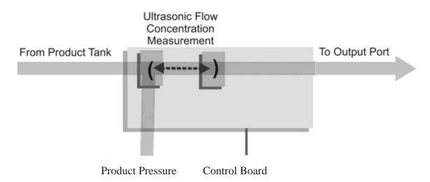
Figure 2: Flow Sensor Board Diagram
