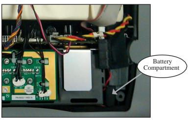
Figure 17: Removing the 9-volt Battery
