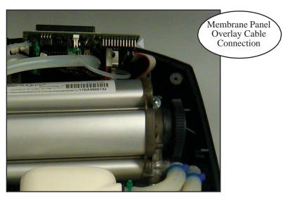
Figure 14: Removing the Membrane Panel Overlay Ribbon Cable.
