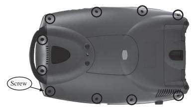
Figure 12: Removing screws to open the Front Cover
