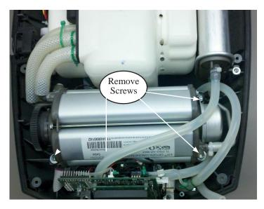
Figure 33: Remove ATF Module from Eclipse 5 Case.
