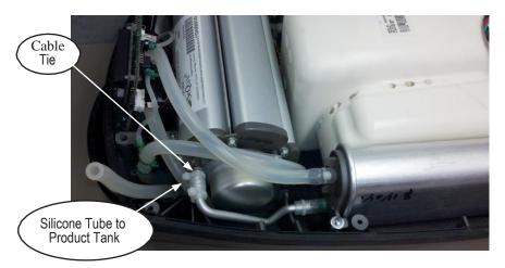
Figure 31: Removal of ATF Module Product Hose.
