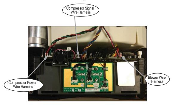
Figure 56: Compressor Box electrical connections.
