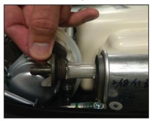
Figure 21: Unscrewing the HEPA Filter.
