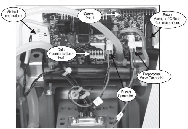
Figure 46a: Control Board Connector Diagram 3 LED Model
