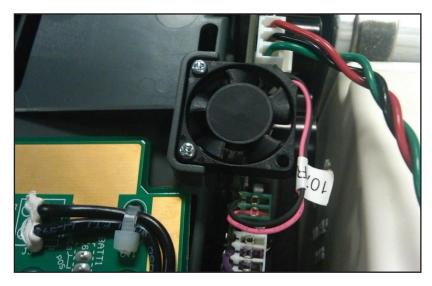
Fig 53: Cooling Fan placement
