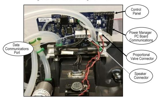
Figure 46b: Control Board Connector Diagram 2 LED Model
