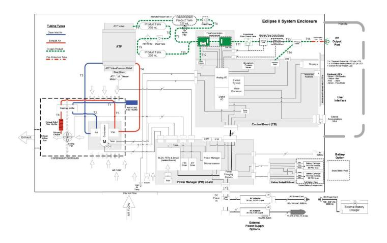
Figure 28: Eclipse 5 Oxygen System Simplified Block Diagram.
