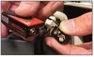
Figure 18: Disconnecting the 9-volt Battery.
