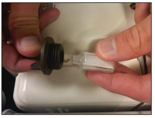
Figure 22: Installing the new HEPA Filter.
