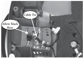
Figure 44: Bonding the Buzzer to the case.
