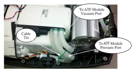
Figure 32: Removal of ATF Module Pressure and Vacuum Tubes.
