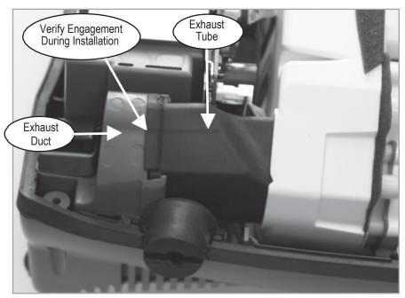
Figure 57: Exhaust Tube Removal.
