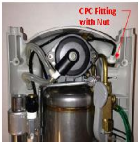
Figure 3. Older Style HELIOS with Check Valve, Tee, and CPC Fitting with Nut.
