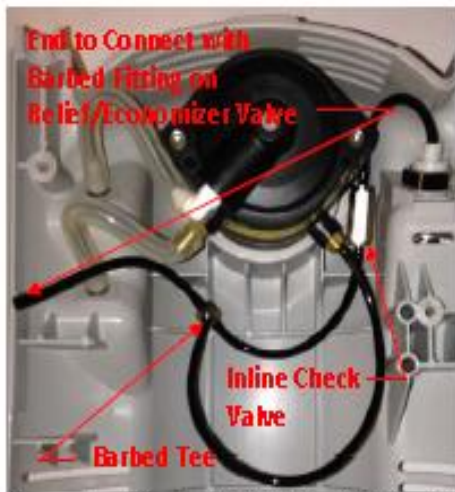
Figure 5. Older Style HELIOS with Check Valve, Tee, and CPC Fitting with Nut (Some components removed and tubing rerouted for clarity).
