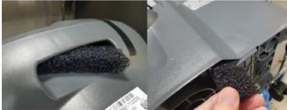
Figure 2: Top Gross Particle Filter (left) and Bottom Gross Particle Filter (right).
