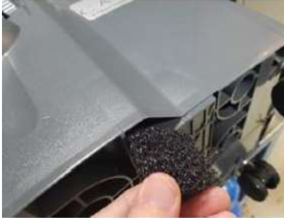
Figure 5. Bottom Gross Particle Filter. Located in front of compressor intake on bottom of unit.
