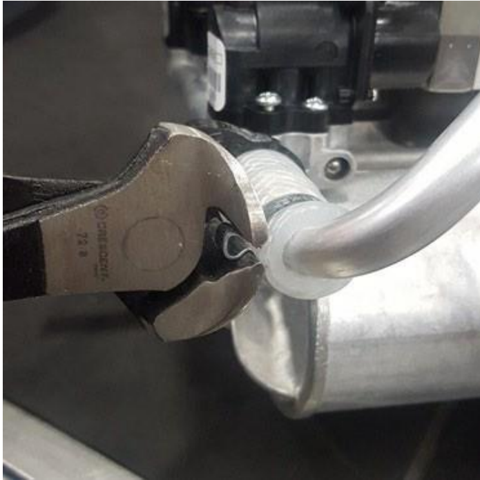
Fig. 5: Crimping Pinch Clamp
