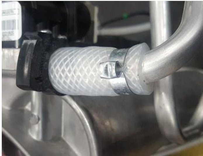
Fig. 6: Pinch Clamp Installed
