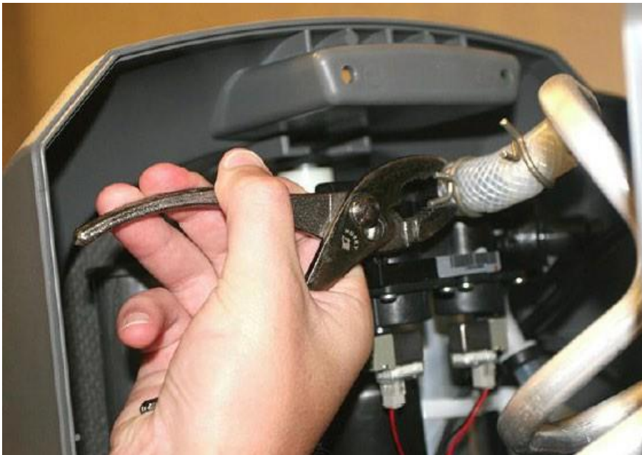
Fig. 4: Precious Design Clamp Removal
