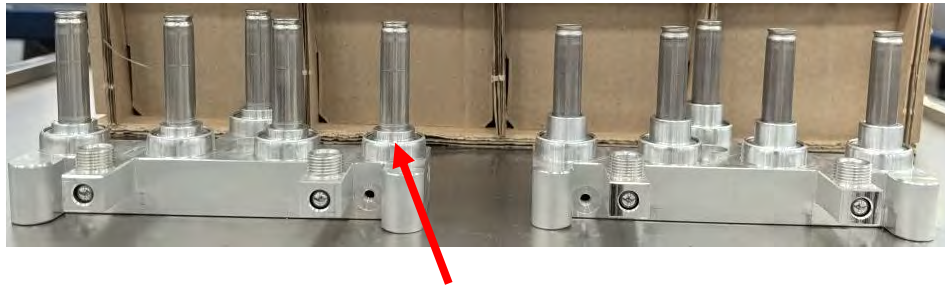
Left side manifold shows a longer stem and a reduction on the valve seating. Figure 1.
