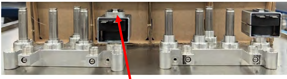
Left side manifold shows valve fitted with washer HA197-1 and secured with clip. Figure 2
