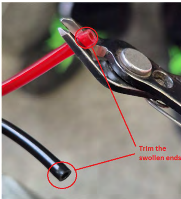
Figure 2 – Trim tubing 3/8" (9mm)
