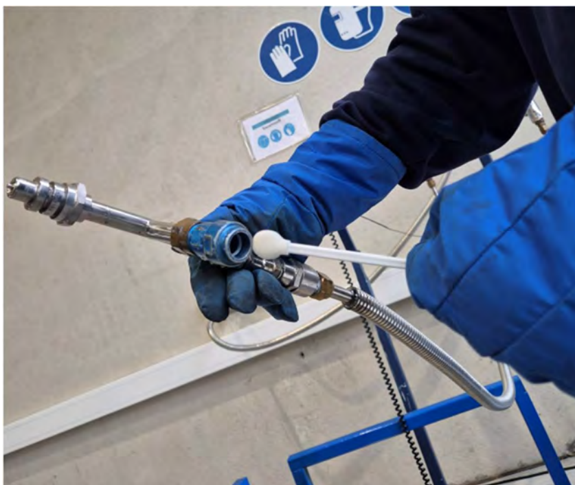
Figure 7 – Wiping of fill connectors depending on QDV Fitted.
