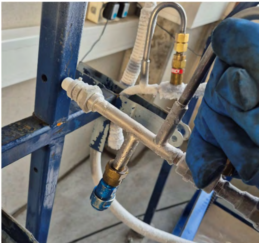
Figure 5 – purging transfer hose.
