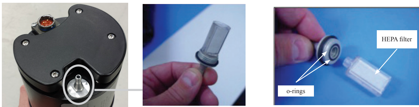
Figure 6-4. Reinstall O2 Fitting/HEPA Filter
