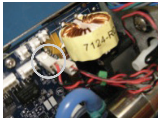
Figure 11-24. Remove Compressor Fan wire
