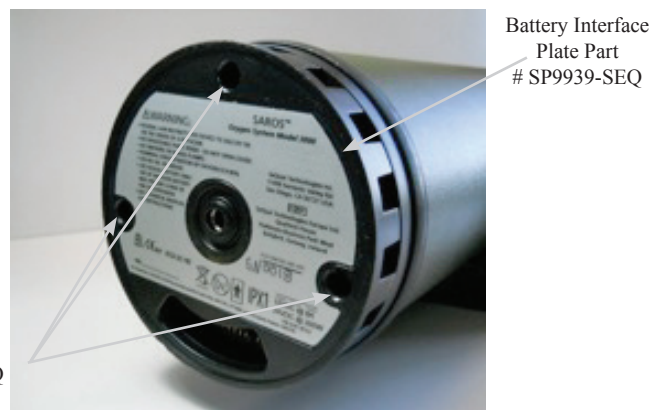
Figure 11-2. Removal of the three BIP screws
