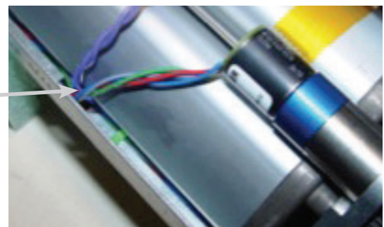
Figure 11-50. Route ATF wires
