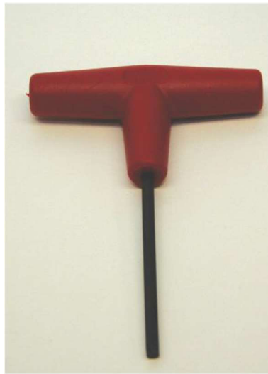
Figure 8.1b 5/32-inch Allen-head driver
