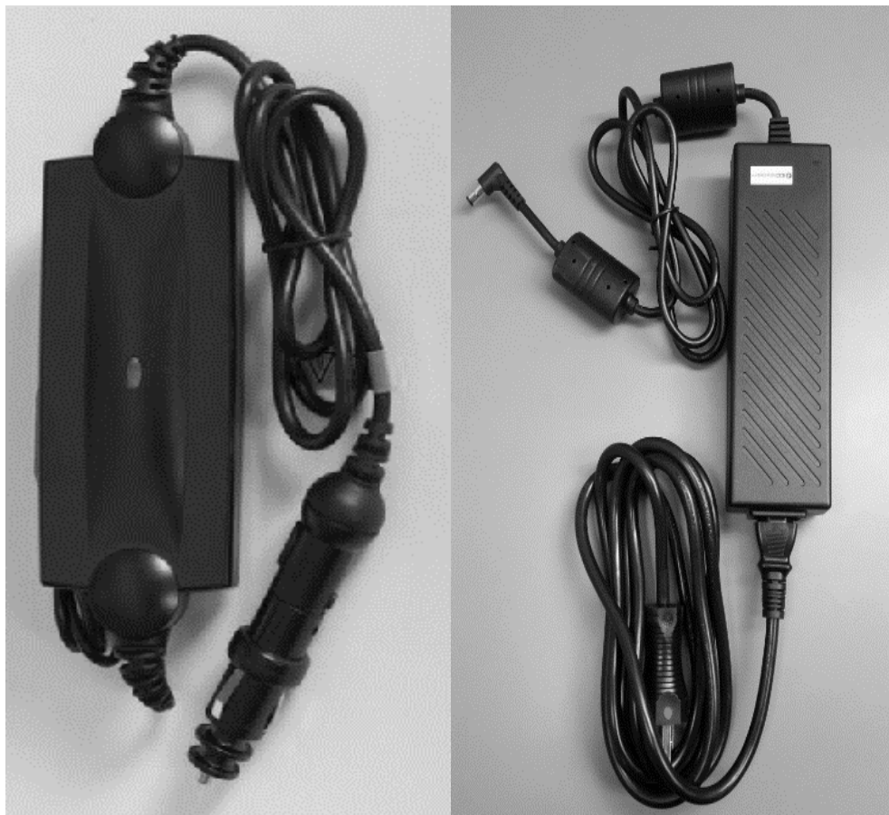
Figure 7: FreeStyle 5 DC and AC Power Supplies
