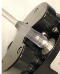
Figure 4-2. Installation de la canule
