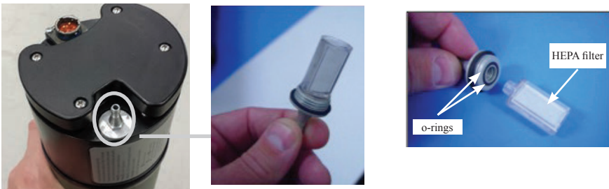
Figure 5-4. Reinstall O2 Fitting/HEPA Filter
