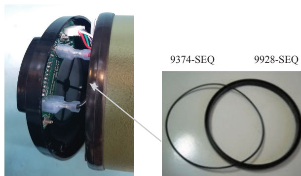
Figure 7-5. Removal of Sleeve Alignment Ring
