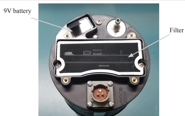
Figure 7-8. Filter Screen and 9V Removal
