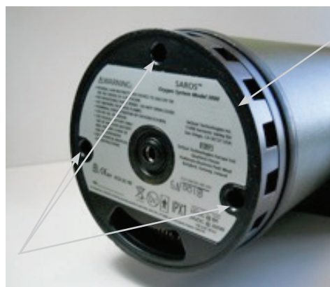
Figure 7-2. Removal of the three BIP screws
