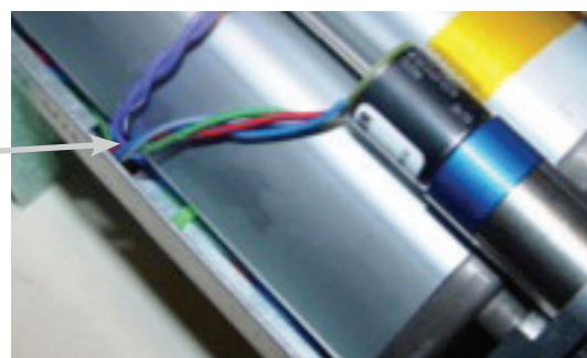
Figure 7-50. Route ATF wires
